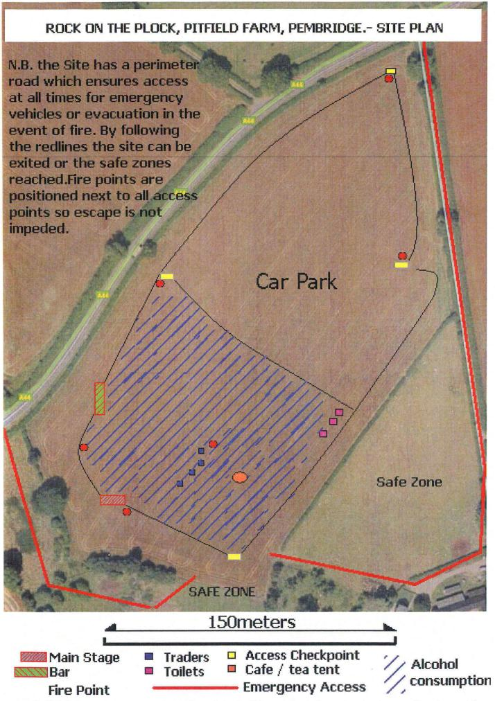
Each F.P. has a flag so its clearly visible. All points includes a bucket of sand and a Co2 fire extinguisher. Fire points by the traders and the bar include a fire blanket aswell.
